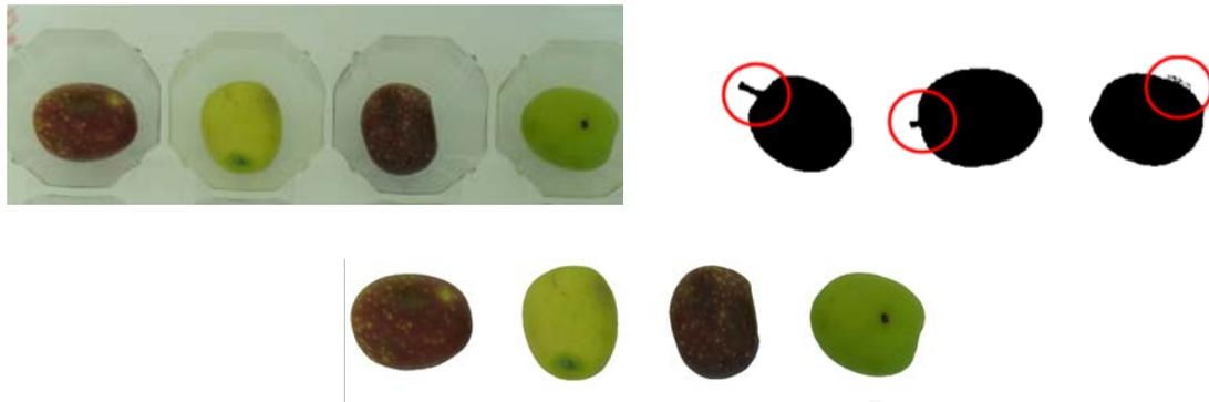
**Figure 2.** (Left) Original images of a group of olives inside a tray; (Right) Black/white image with three defective olives. (Bottom centre) Final segmentation of group olives.
