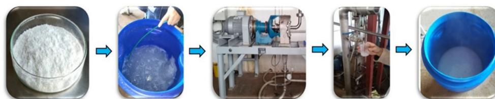
**Figure 10.** Processing of NF  $\beta$ -chitin at bench scale using a massive collider machine.
